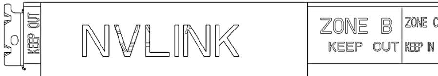
Sufficient clearance must be provided both above the card's north edge and behind the backside of the card's PCB to accommodate NVIDIA A100 80GB NVLink bridges. The clearance above the north edge should meet or exceed 2.5 mm. The backside clearance (from the rear card's rear PCB surface) should meet or exceed 2.67 mm. Consult *NVIDIA Form Factor 5.0 for Server Cards* for more details.
